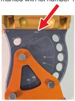
2. Using a 3/8 hex wrench, remove the four large bolts securing the Half Plate Assembly to the Main Plate.
